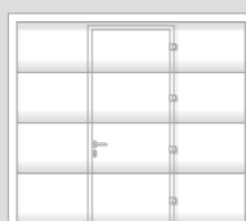
Symmetrical arrangement for garage door widths up to 3,500 mm
